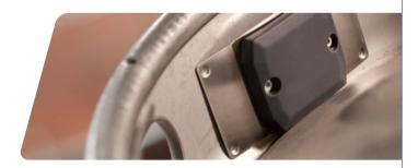
When the application is too demanding for adhesives, but the metal surface cannot be punched for screw or rivet fixing, welding the tag with special bracket is an option for attachment. Welding bracket is made of stainless steel and allows attachment on both flat and curved surfaces.
