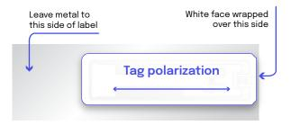
Minimum bending diameter of the **Beontag Silverline Micro II** is 100mm. For optimal performance please bend the label in the orientation shown below.
